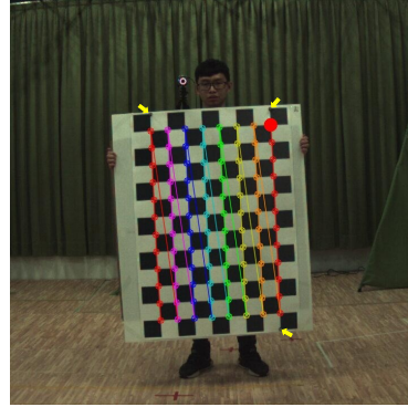
Listing 1: Compute the rigid transformation Fig. 2: One image with pattern drawn for camera calibration
